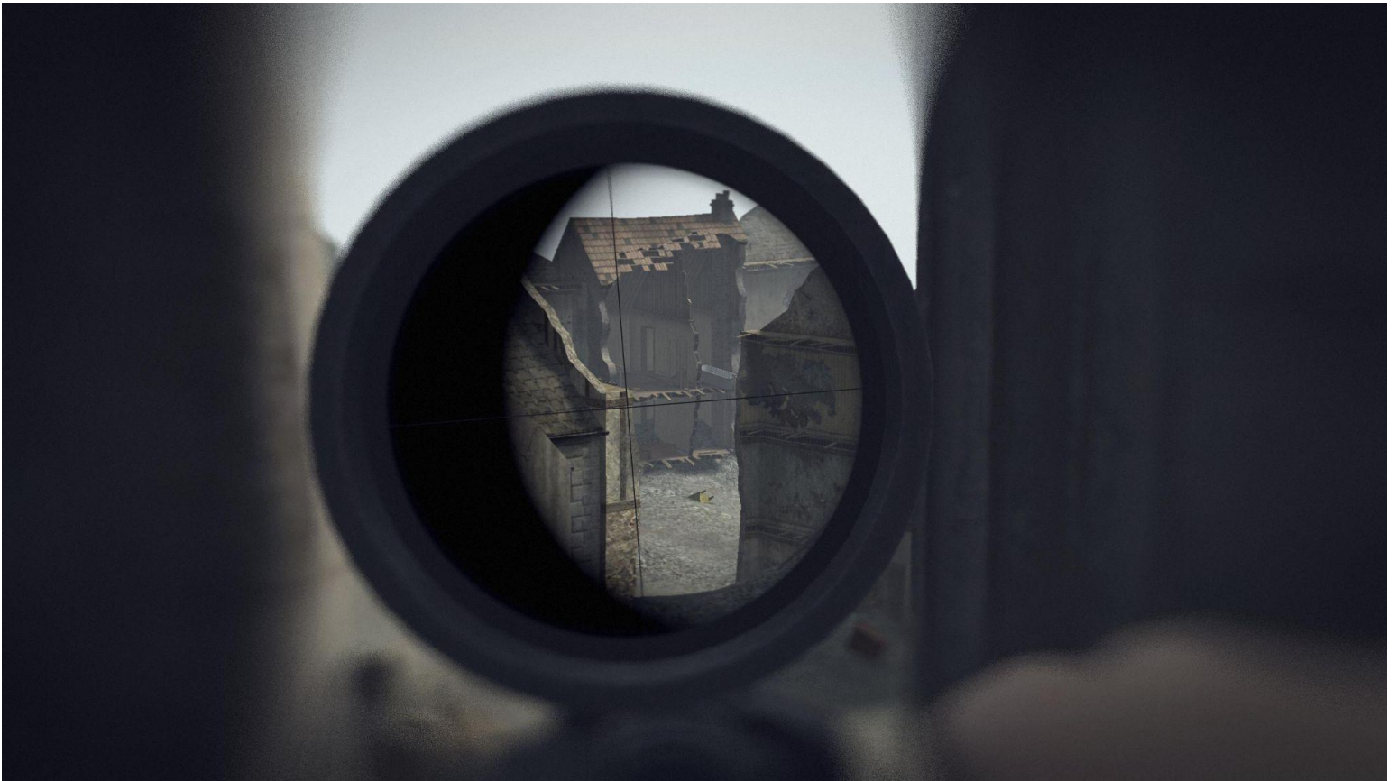
Figure 3. - Scope Shadow as seen on U.S. rifle, caliber .30, M1903A4 while bolting the action.
